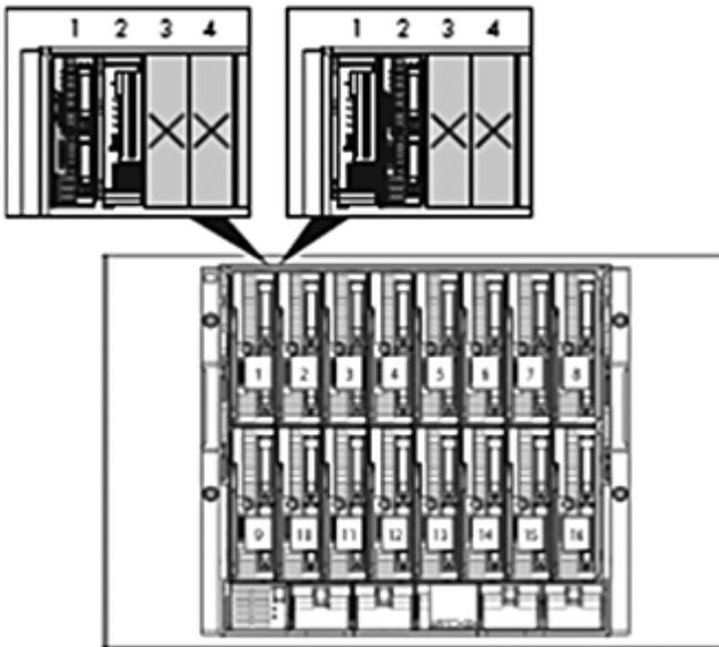
**Figure 1** Installing a tape blade adjacent to a half-height server blade in a c7000 enclosure.
